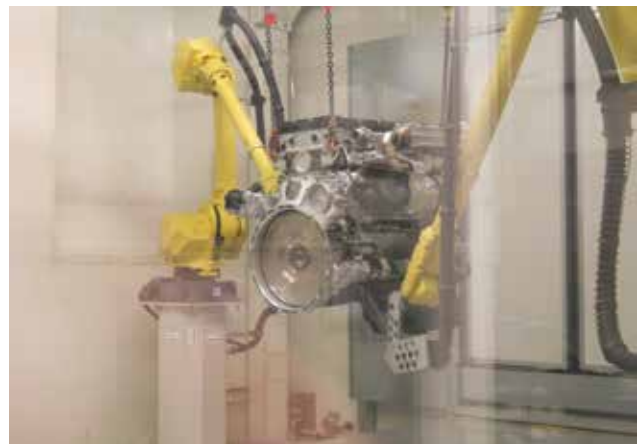
Cleaning of heavy duty diesel engines using CO 2 pellets, Source: Daimler AG
