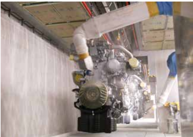
Painting of heavy duty diesel engines, Source: Daimler AG
